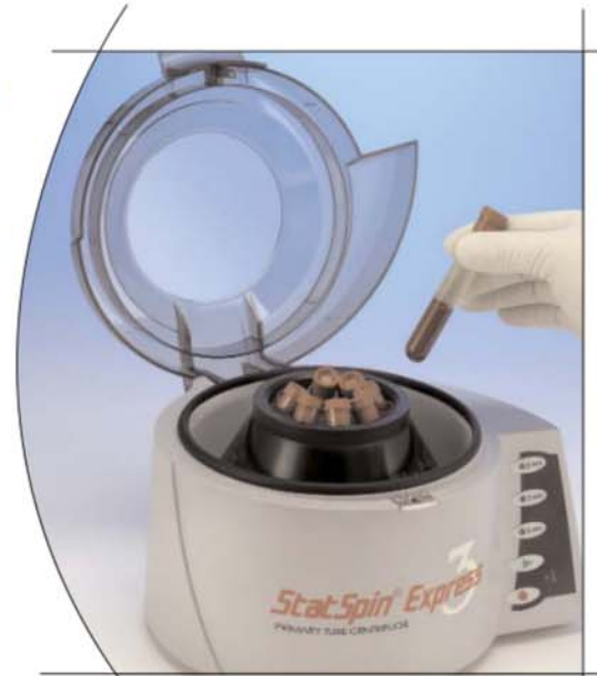
The StatSpin Express 3 holds 8 tubes up to 10 mL.
